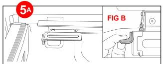
Position the rail with the silver, slotted bracket all the way forward, towards the cab, front of the vehicle.
