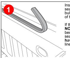
Install the bulkhead seal to the top of the bulkhead at the edge of the bed opening.
